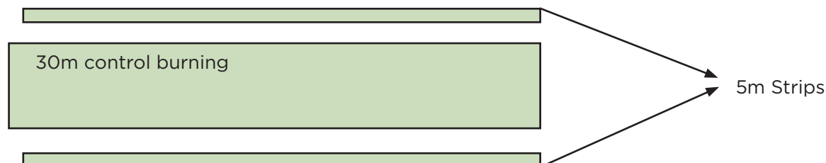
FIGURE 6. 3 : DIAGRAM SHOWING CONTROLLED PRE-BURNING AND STRIP BURNING
